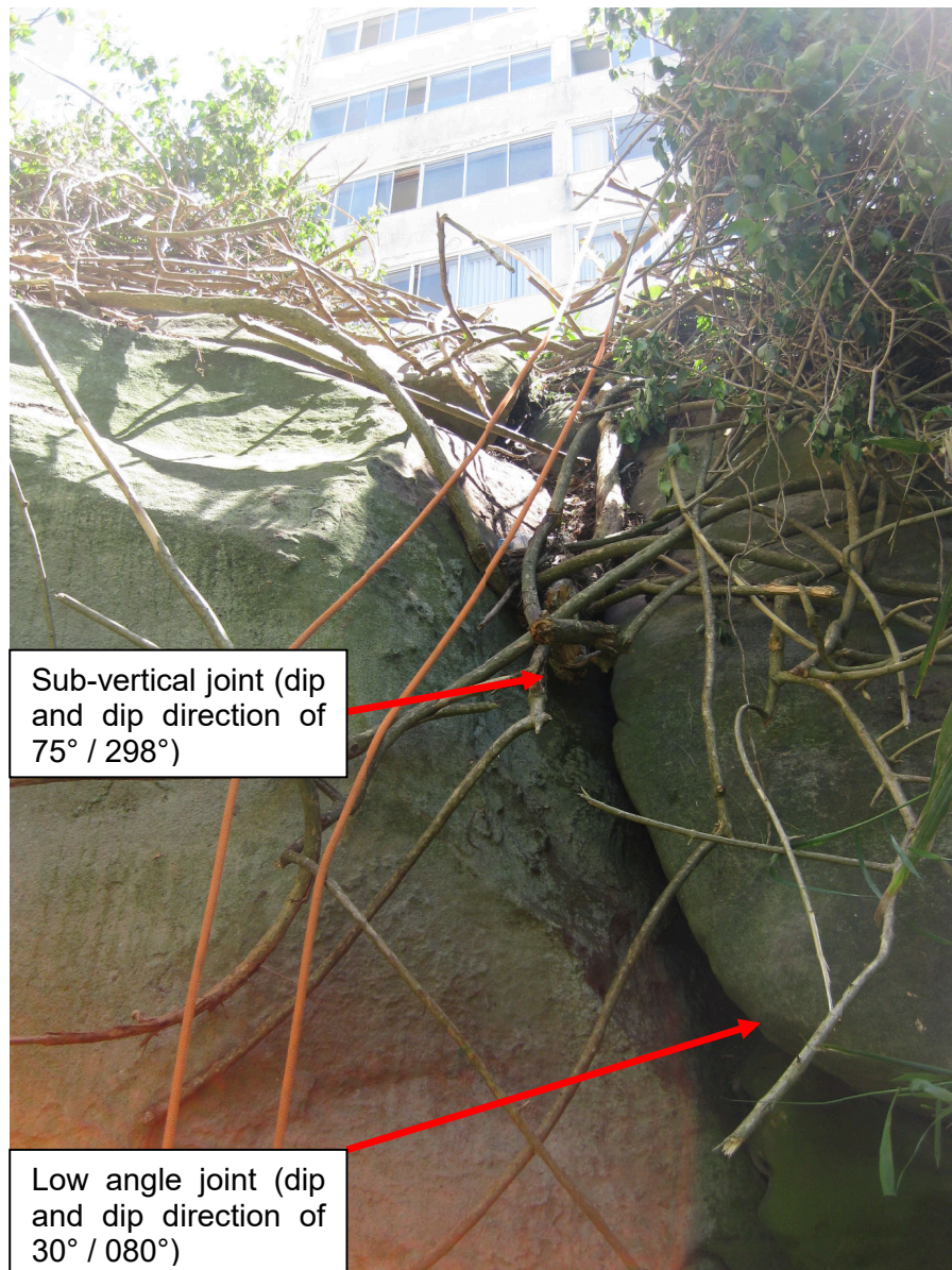
Mapping Traverse 107, Photo 3 – View upslope from base of traverse 107, of sub-vertical and inclined joints within a bed of massive sandstone. The joints and their orientations are indicated as shown.
