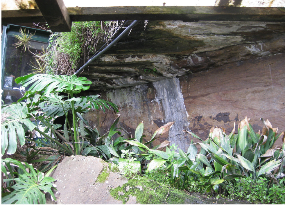
Mapping Traverse 102, Photo 4 – View of overhang in cross-bedded sandstone (RL47.5 m) at mapping traverse 102, with a sub-vertical, iron-stained joint plane forming the rear of the overhang.
