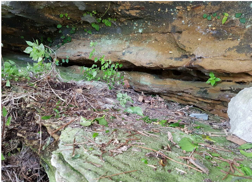
Mapping Traverse 102, Photo 2 – View of a continuous bedding parting defect and overhang (cave) at mapping traverse 102, with a sub-vertical, iron-stained joint plane forming the rear of the 'cave'.
