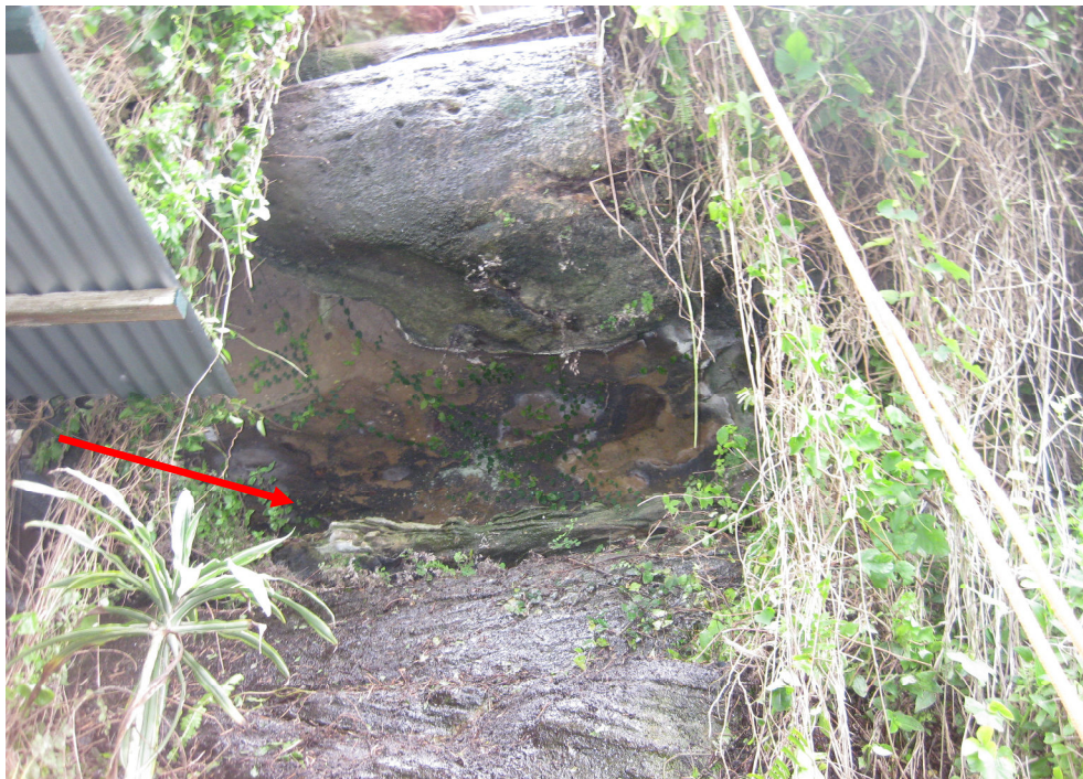
Mapping Traverse 102, Photo 3 – View of overhang at RL51 m on mapping traverse 102, with a bed of massive sandstone above and cross-bedded sandstone below. Cave location is indicated as shown.
