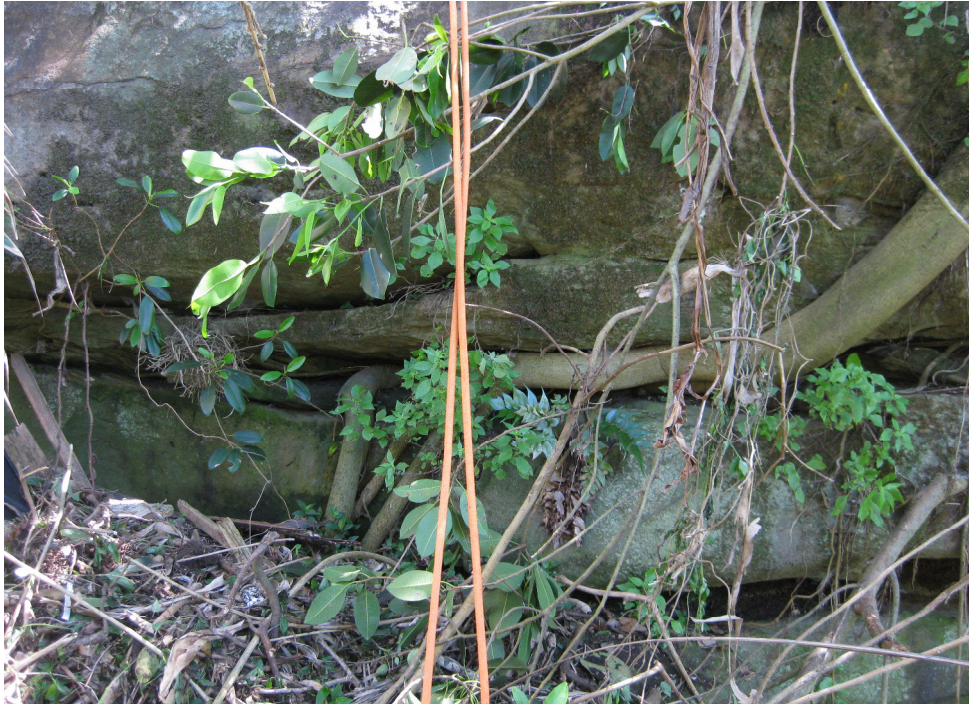
Mapping Traverse 106, Photo 3 – View of base of cliff at mapping traverse 106. Fig tree roots and evidence of past seepage were observed within small caves and overhangs formed in cross-bedded sandstone.
