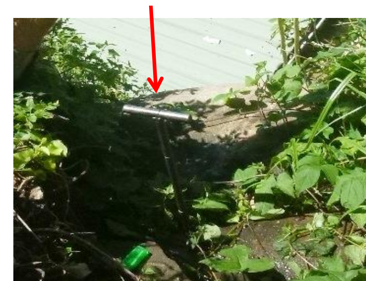
Photo 8a. Close up of test probe inserted into the open joint.
