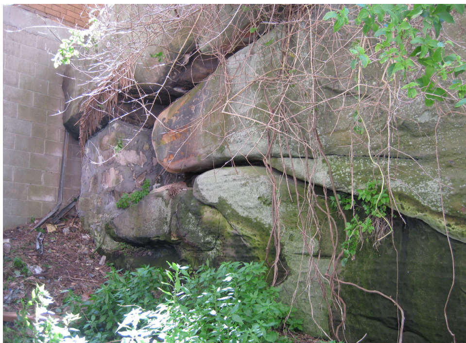
Mapping Traverse 109, Photo 2 – View north towards mapping traverse 109, showing sub-horizontal and dipping bedding plane defects.
