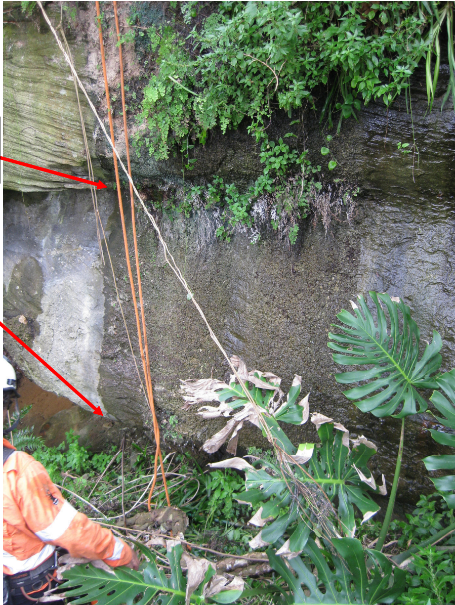
Mapping Traverse 101, Photo 3 – View of lower portion of slope along mapping traverse 101. High strength cross-bedded sandstone exposed, and with an overhang formed above a bedding parting defect which extends more than 10 m to either side of the section line.
