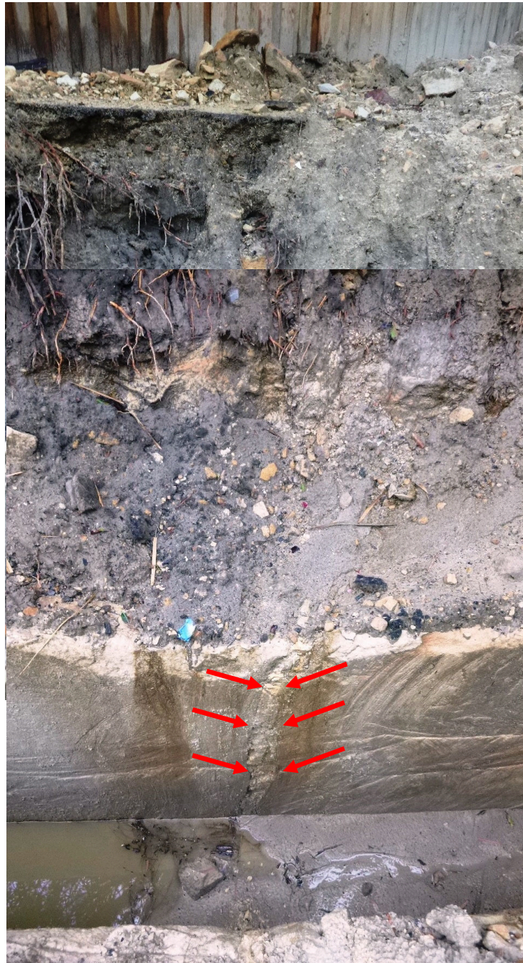
Historical Site Photograph of Sewer Diversion Trench, Photo 4 – View to north-west near Borehole BH5 and BH103. Sub-vertical, clay-infilled undulating defect in rock (indicated between arrows as shown), inferred to be an intrusive dyke weathered to clay, or a clay-infilled joint defect.
